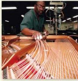
Treble strings are made of high-quality steel, and bass strings are made of copper-wound steel strings. The strings are all uniformly spaced with one end coiled around the tuning pins, which in turn are inserted in a laminated wooden block called the pin-block or wrestplank.
